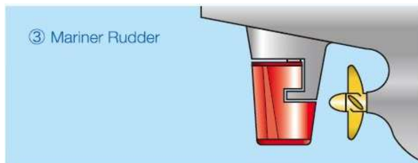
Gambar 7. Kemudi setengah menggantung ( Marine rudder ) (Omdaka Bldg. (2003). The Fish Tail Rudder. Tersedia: http://www.japanham.com/en/service/schilling/ )
