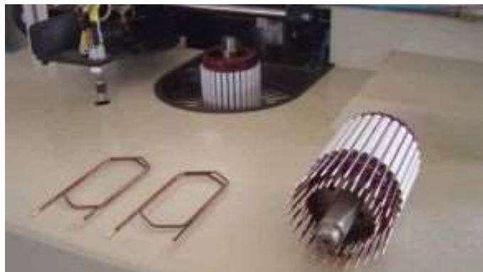
Gambar 5 Armature Winding Conductor
