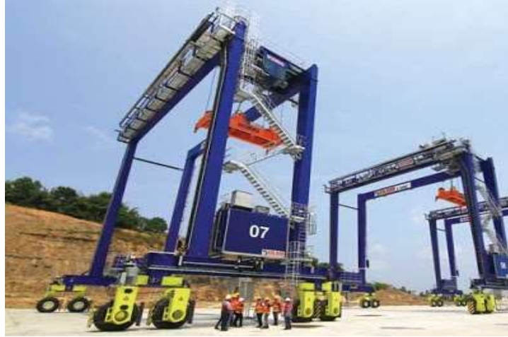
Gambar 4. Rubber Tyred Gantry Crane ( RTGC )
