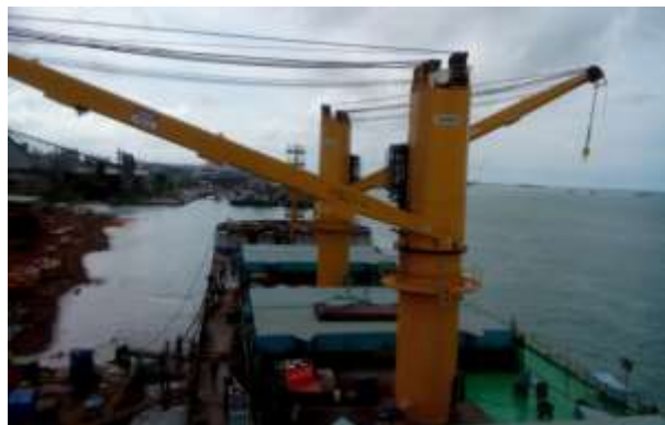
Gambar 1. Crane kapal (ship gear)
